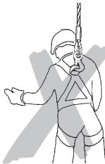
Only units fitted with hooks with safety latches must be suspended in the eye. Make sure that the hook is not too large. The eye must be seated centrally in the saddle of the hook and the hook must be freely articulating in the eye.
