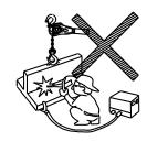
Do not perform welding or cutting operation on the load being suspended.
