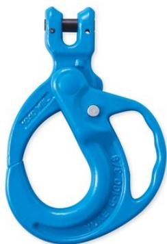
Proof Load tested at 2.5 times the WLL with certification for each batch manufactured. Fatigue rated to 20,000 cycles at 1.5 times the WLL. Magnaflux crack detection is performed 100% on each batch.
