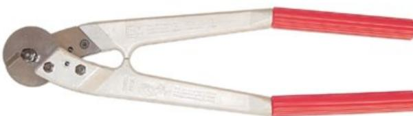
Cut both hard-drawn wire like steel-, copper- and aluminum wires, electric cables and multi wire ropes. The cutting edges are shaped to form a grip of the rope, in shape of a triangle when cutting which prevents un-twisting of the rope end. The edges are made in alloy steel of coromanttype. The cutters are provided with plastic handles.
