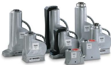
Aluminium jacks combine lightweight with high lifting capacity. The use of high tensile aluminium alloy allows lifting capacities of up to 100 tonne resulting in a very favourable 1.8 tonne lifting capacity per 1kg weight ratio.
