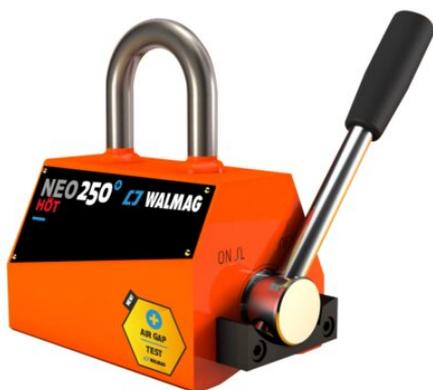
The Neo HOT permanent lifting magnet is designed for a long life span even in the most demanding operations at working temperatures up to 180°C. Its design makes it possible to handle flat and round load profiles. The high lifting capacity is achieved by using a double magnetic circuit of strong neodymium magnets.
