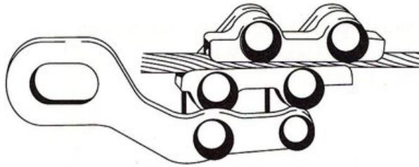
**General:** For safe and careful installation, tensioning or pulling of ropes. The tension spring construction allows to position the clip on the rope without any additional fixing and maintains the grip on the rope even if the rope is unloaded.
